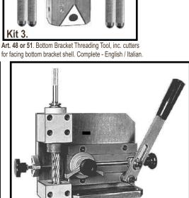
Machine for Milling Brake Bridge. Holders for different Bridges available.
